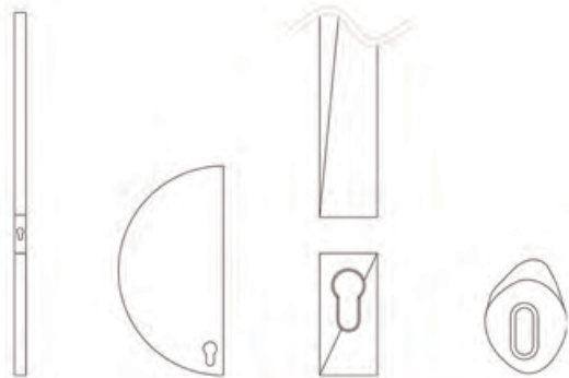
1000 pull handle 1000 x 34mm 300 D handle 300mm escutcheon 65 x 34mm woodland escutcheon 65 x 45mm
